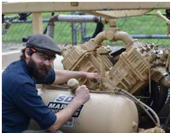
Kurt is working on a diesel-powered air compressor which supplies air to the divers. It can also be used to pressurize the hyperbaric chamber used to treat decompression sickness.
