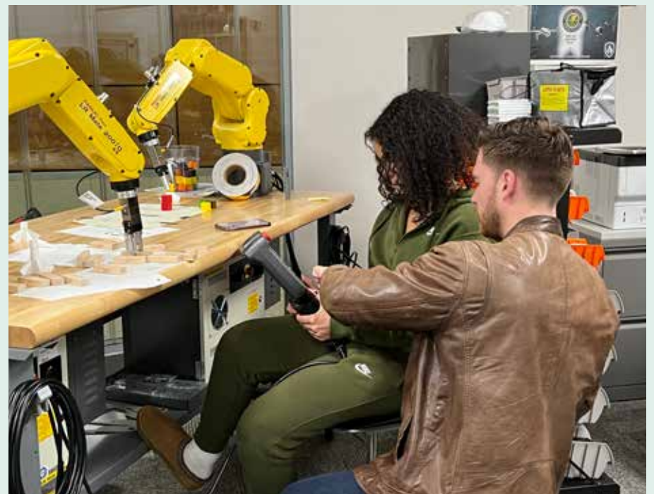
Dillon Lippman, an Electrical Engineering Bachelor of Science degree student and a lab assistant/peer tutor, demonstrates to a Pawtucket student how to use a programming pendant to move/program the FANUC robotic arm which can move items/products from one place to another as well as paint, weld, and assemble them.
